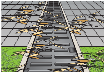
In agricultural areas small particles, such as straw, silage, etc. can get stuck in the slots of the mesh grids.
